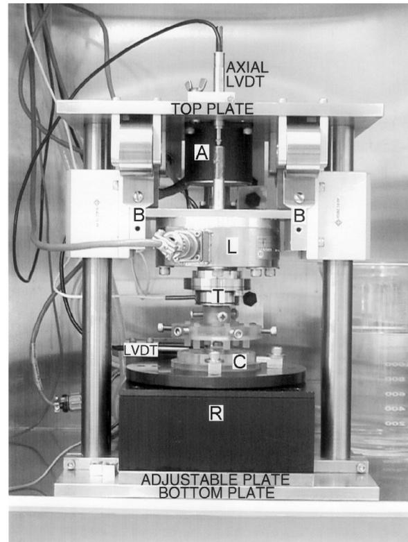
Fig. 1. Shear/compression apparatus: A — axial linear stepper motor; B — bearing/carriage assembly; C — sample chamber; L — load cell; T — torque cell; R — rotary position table. The adjustable plate may be moved to accommodate other fixtures. The LVDT shown to left of chamber (C) senses rotational displacement. Rotary table (R) is driven by stepper motor behind the table.
