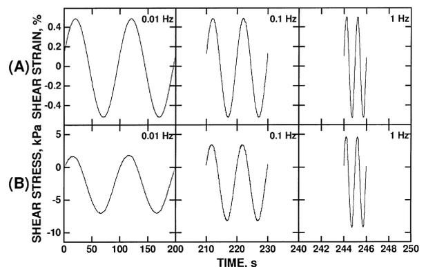
Fig. 3. Examples of (A) applied sinusoidal shear strain, and (B) resulting stress waveforms at 0.01, 0.1 and 1 Hz for 4 articular cartilage disks tested simultaneously in the chamber of Fig. 2 (spaced symmetrically at  $90^\circ$  apart). The time axis is expanded in middle and right panels to show details. Shear stress waveform indicates an increase in shear modulus with frequency. The phase angle of stress relative to strain was approximately  $10^\circ$  at all 3 frequencies.
